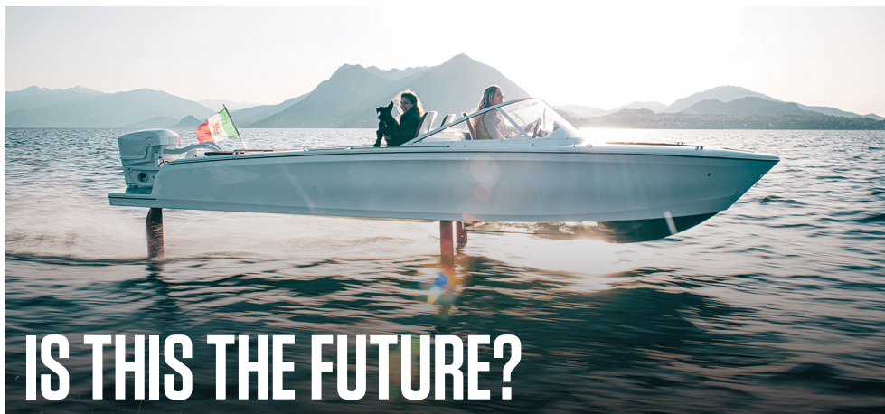
Photo: Courtesy of Candela. Candela ® C-7 cruising over 20 knots on computer controlled hydrofoils. GBF notes there continues to be many innovations in high-speed electric boats to deal with battery power/size required and this is just one example.
