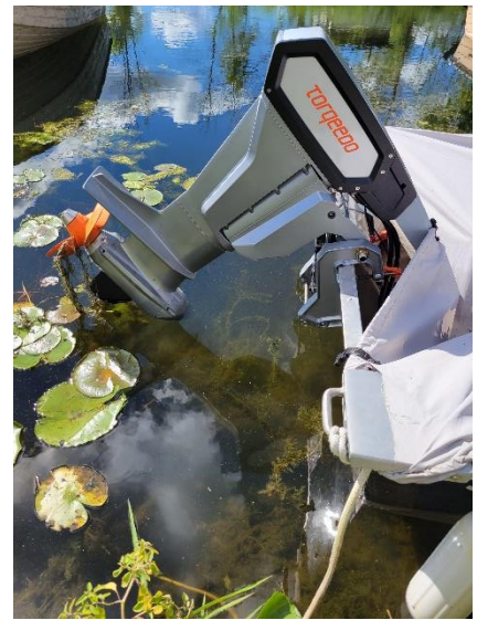
Figure 3: The 20HP fully electric outboard motor, manufactured by Torqeedo.
