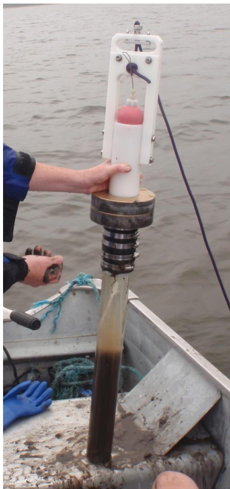
Photo 1. Core Collection Apparatus with Sediment Core
